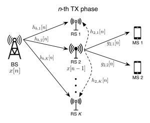
Fig. 1. A two-hop single-cell downlink network with K half-duplex relays.
