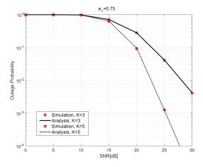
Fig. 3. Comparison simulation of outage probability of the proposed protocol with analysis when  $K=3,\,\kappa=0,\,R_1=0.5$  bits/s/Hz and  $R_2=2$  bits/s/Hz for 20 phases.
