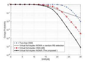
Fig. 4. Outage probability comparison between the OMA and NOMA based schemes when  $K=5\ (R_1=0.5\ {\rm bits/s/Hz}$  and  $R_2=2\ {\rm bits/s/Hz}).$
