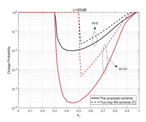
Fig. 9. Outage probability according to  $a_1$  when  $\rho=20$  dB ( $R_1=0.5$  bits/s/Hz and  $R_2=2$  bits/s/Hz).
