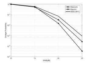
Fig. 6. Outage probability of the proposed technique according to beamforming technique when the number of antennas at the BS is equal to  $5\ (M=5)$ .
