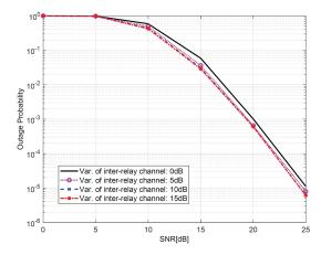
Fig. 7. Comparison of outage probability according to the inter-relay distances when K=5 and  $a_1=0.75$ .
