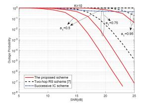
Fig. 5. Outage probability for varying SNR values when  $K=10\,$  ( $R_1=0.5~{\rm bits/s/Hz}$  and  $R_2=2~{\rm bits/s/Hz}$ ).
